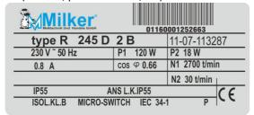
machine (the model, serial number, year of manufacture, refrigeration capacity in Watt, electrical power in Watt, voltage, refrigerant type and quantity) and the CE mark.
